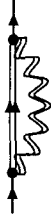
Fig. 16.9 Diagrammatic representation of the self-energy in the ring approximation, known as the GW approximation. The screened Coulomb interaction W is represented by the double wiggle and consists of summing all rings that contain the dressed sp propagator G , shown as the double line.
