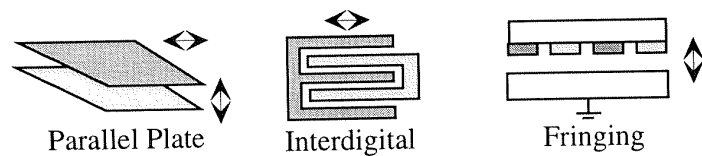
Figure 19.3. Illustrating a variety of capacitor structures that can be used for position sensing.
