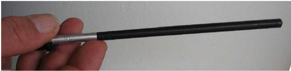
FIG. 12. 100 mm long CT ionization chamber. This chamber is commonly used for assessment of CTDI.
