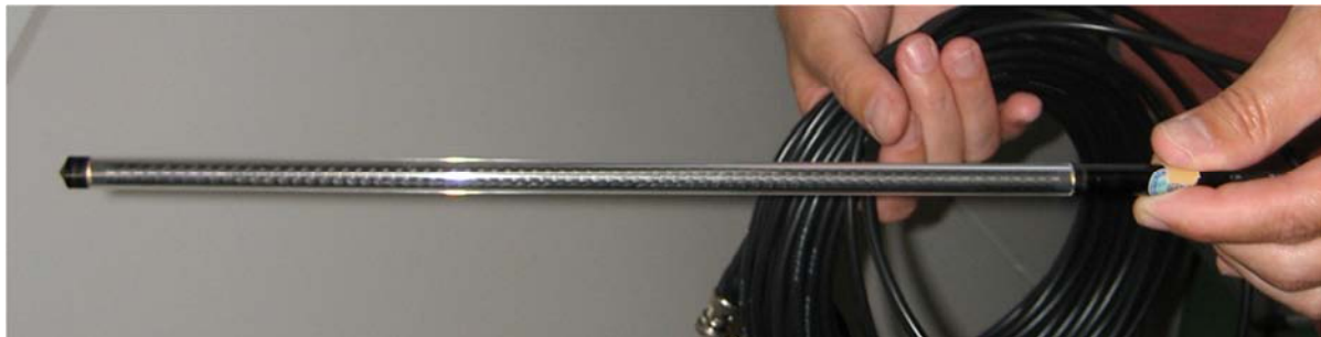
FIG.13. 300 mm long CT ionization chamber, sometimes used, mainly for research purposes.
