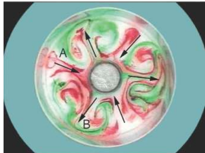
Figure 8.7: Top: Baroclinic eddies in the “eddy” regime viewed from the side. Bottom: View from above. Eddies draw fluid from the periphery in toward the centre at point A and vice versa at point B. The eddies are created by the instability of the thermal wind induced by the radial temperature gradient due to the
