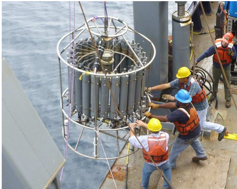
Figure 43: A rosette of sampling bottles with CTD sensors also attached to the rosette frame.
