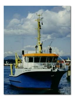
F/F Trygve Braarud is the biggest sea-going vessel of UiO. It is a floating laboratory with modern sensors for measuring physical, chemical and biological parameters. Its normal region of operation is the inner and outer Oslo fjord. F/F Trygve Braarud, built in aluminum, was constructed in 1983 at Linstøls Skips- og Båtbyggeri in Risør, Norway. The vessel is 21,8 m long, has a normal cruising speed of 9,5 knots (18 km/h) and a maximum speed of 12 knots (22 km/h).
