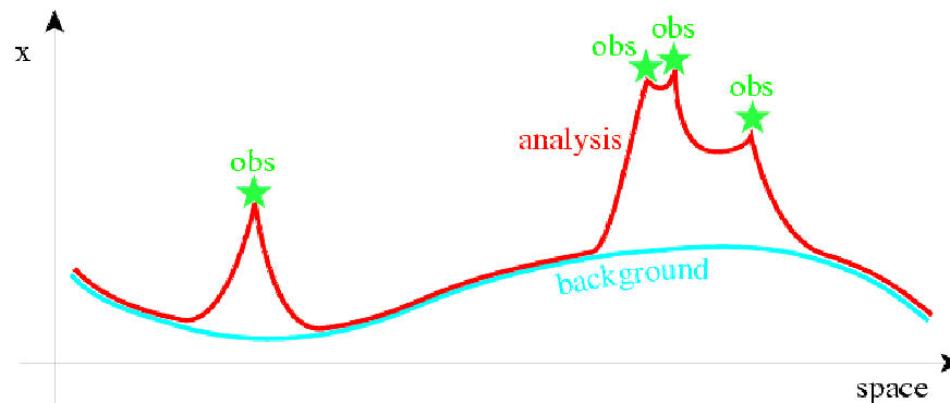
Figure 3. An example of Cressman analysis of a one-dimensional field. The background field x_b is represented as the blue function, and the observations in green. The analysis (black curve) is produced by interpolating between the background (grey curve) and the observed value, in the vicinity of each observation; the closer the observation, the larger its weight.
