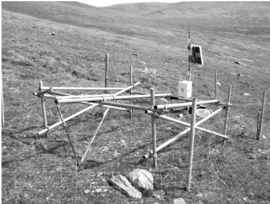
Figure 2 The Steinhøi monitored solifluction lobe showing the frost heave frame, with the LVDT fixed base triangle in the foreground and logger box and solar panel in the background. The apex of the LVDT triangle is attached to a footplate embedded in the ground surface (see Harris et al. , 2007, for details). Thermistors measuring air temperatures are shielded with white plastic tubing and attached to the solar panel pole. The station is fenced against large animals.
