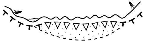
Stage 4a Ice segregation (frost heaving) of alas floor
