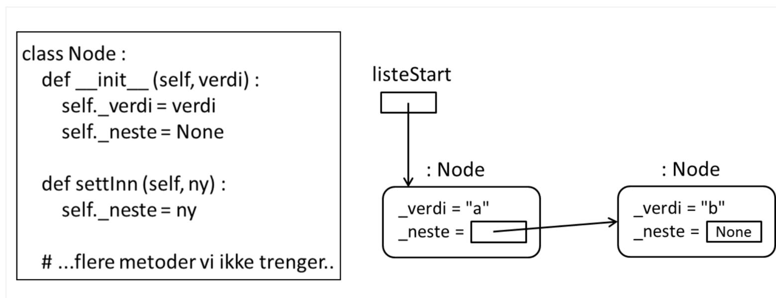
Given the class **Node** shown in the enclosed code, write a procedure **hovedprogram()** which creates 2 objects with values "a" and "b" in a structure as shown in the illustration. The variable **listeStart** (shown as a square) refers to (shown as an arrow) one of the objects. (The objects are shown as rectangles with rounded corners.) You may assume the the class **Node** has been imported to your program.
