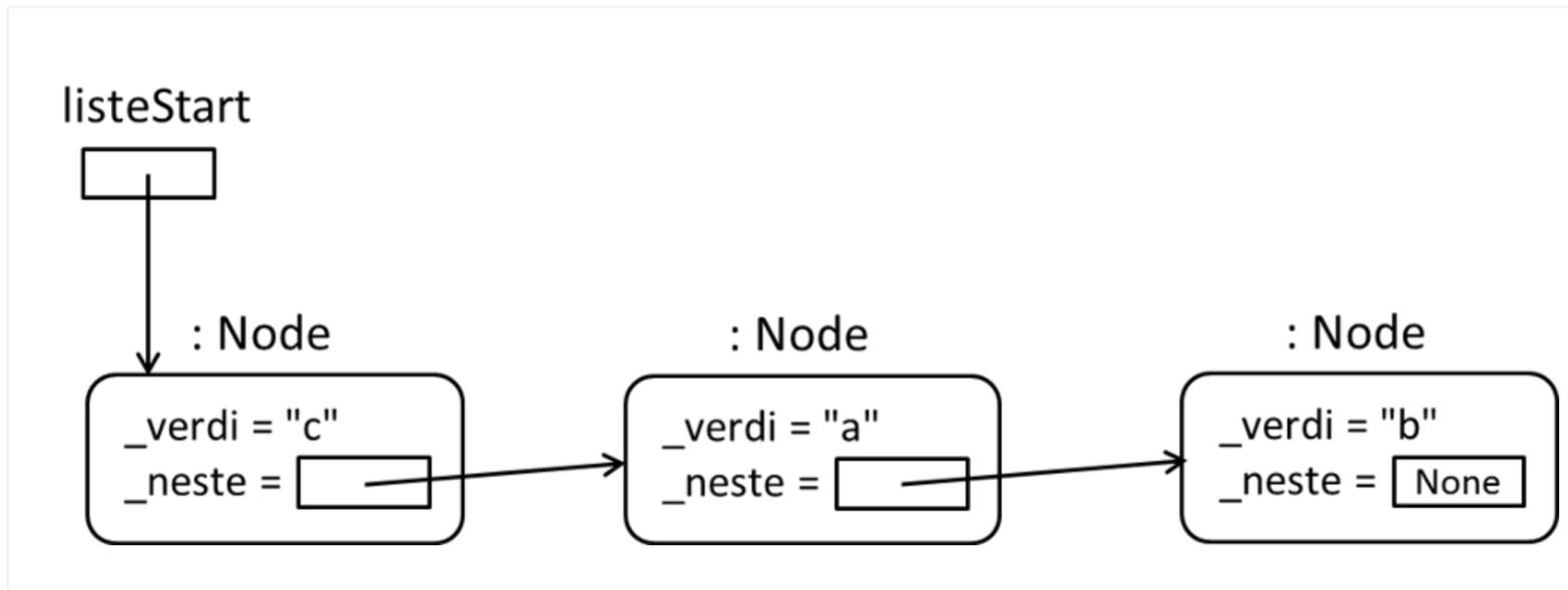
Extend the procedure **hovedprogram** from problem e with code creating another object with value "c" and updates the references to obtain a data structure shown in the enclosed illustration.
