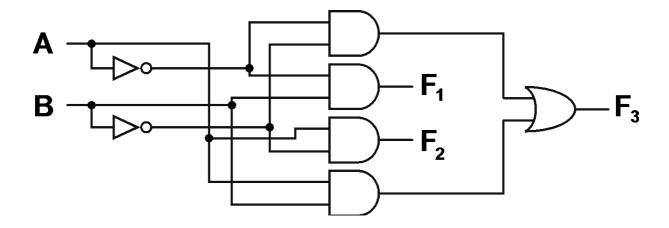
What are the functions (F1, F2 and F3) of the circuit in the figure above? Can you recommend a simplification that contributes to fewer ports.
