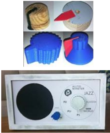
Figure 3. The prototypes for the knob (above) and the digital radio (below). Photo by Johnsen et al. [43].
