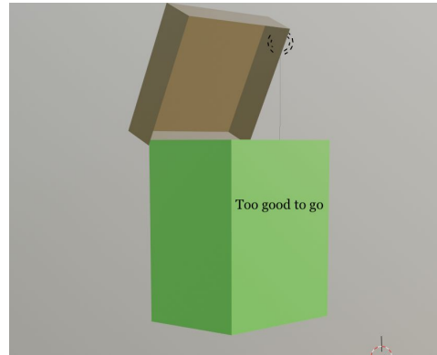
Figure D-11 Second prototype of the box with the lid opening upwards
