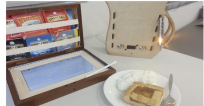
Figure 1 The Kettle Mate and Tea Box. When the connected remote kettle (in another house) is switched on, the kettle mate displays a dynamic orange/red show of lights as shown.
