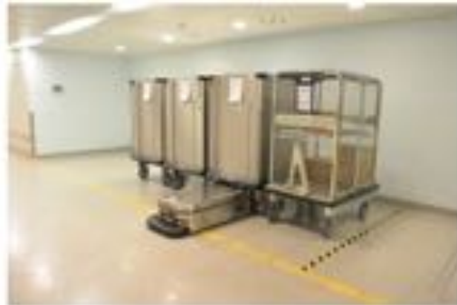
Fig. 2. An AGV picking up a cart
