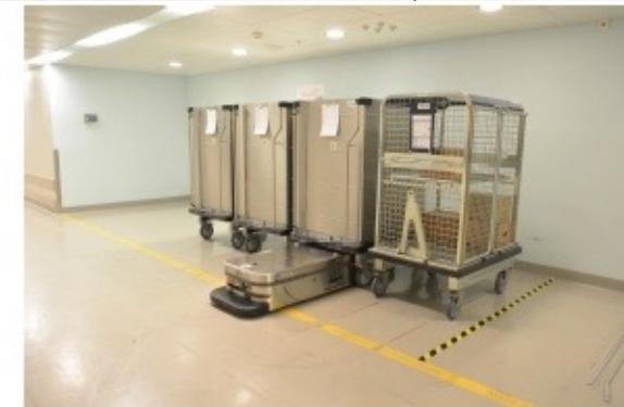
Fig. 2. An AGV picking up a cart
