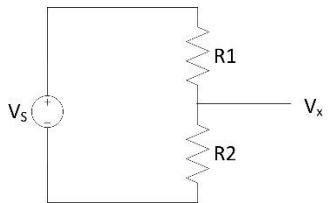
$V_x = \frac{R_2}{R_1 + R_2} V_s$                                                                                                                                               |
