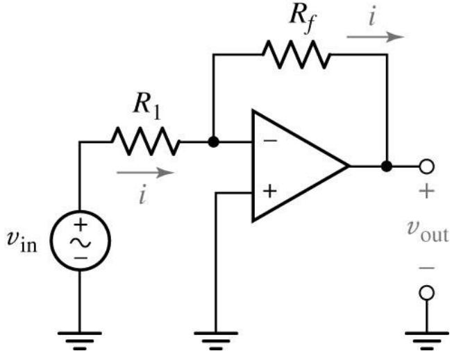
$A_{cl(in)} = -\frac{R_f}{R_i}$ $V_{out} = V_{in}A_{cl(in)}$     |
