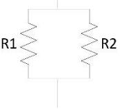
$R_{tot} = \frac{R_1 R_2}{R_1 + R_2} \Leftrightarrow$ $\frac{1}{R_{tot}} = \frac{1}{R_1} + \frac{1}{R_2}$ $\frac{1}{R_n} = \frac{1}{R_1} + \frac{1}{R_2} + \dots + \frac{1}{R_n}$ |
