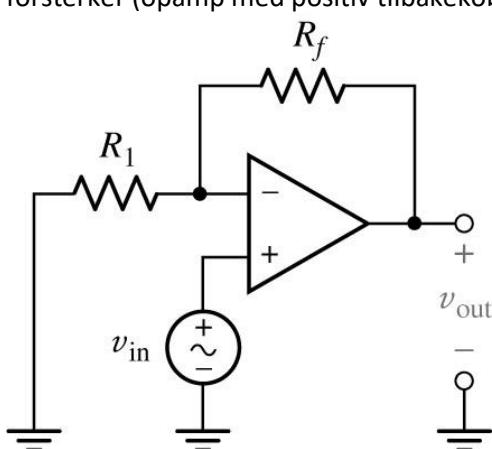
$A_{cl(ni)} = 1 + \frac{R_f}{R_i}$ $V_{out} = V_{in}A_{cl(ni)}$ |
