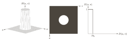
FIGURE 4.40 (a) Perspective plot of an ideal lowpass-filter transfer function. (b) Filter displayed as an image. (c) Filter radial cross section.
