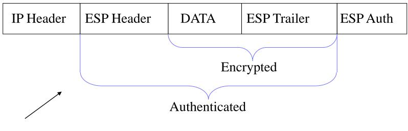
Original IP Packet protected by Transport-ESP
