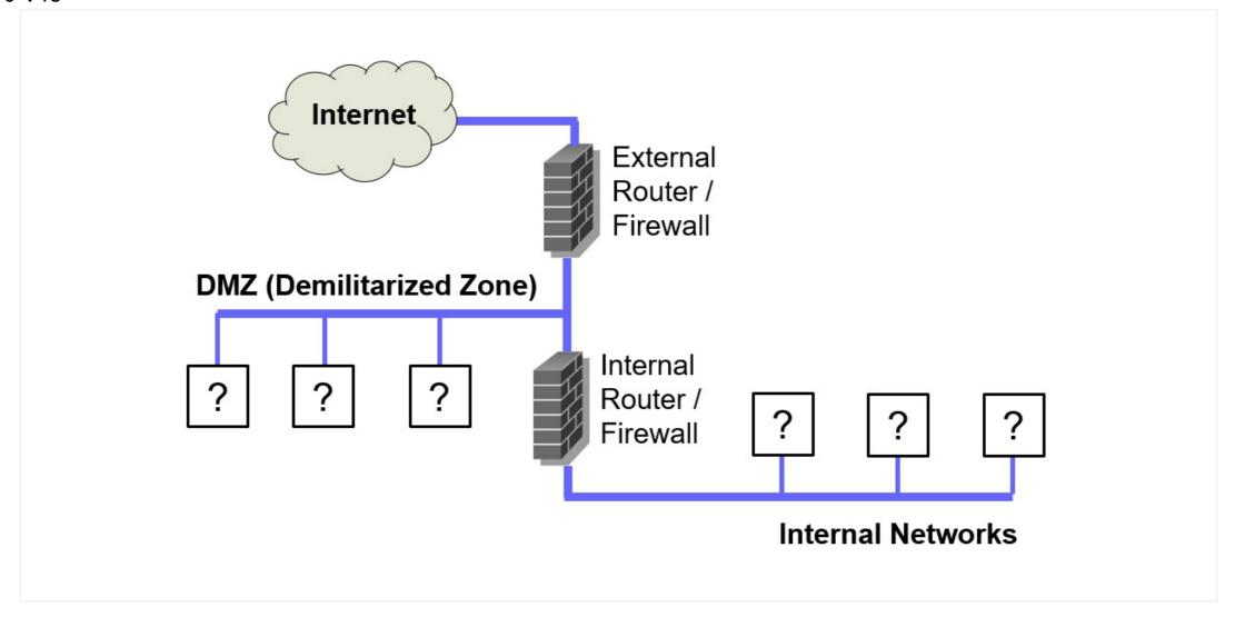
In the case of two firewalls with a so-called DMZ (Demilitarized Zone) between them, servers/systems can be connected to either the DMZ or to internal networks. Select the typical location for connecting the servers/systems in the left column below.
