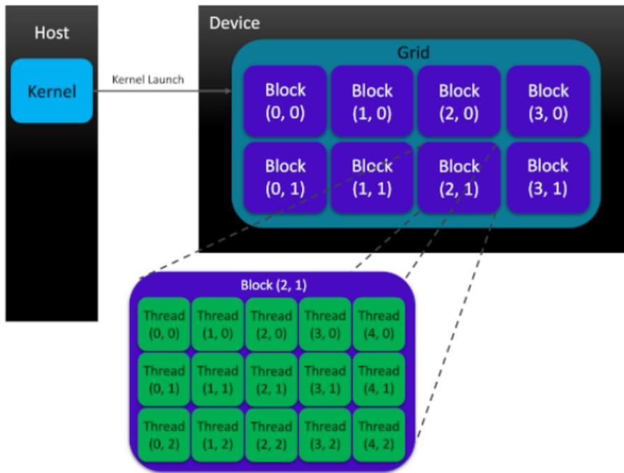
Blocks and Grids have at most three dimensions—denoted x, y, z, with x innermost and z outermost. Their sizes are specified at kernel launch. Inside the **kernel** you may use:
