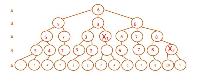
The X1 branch i pruned because a smaller value than 3 is irrelevant as A already has a 5 i the left main branch of the tree (at this point the alphsn value in the root will be 5). A larger value than 3 will never be chosen by B.
