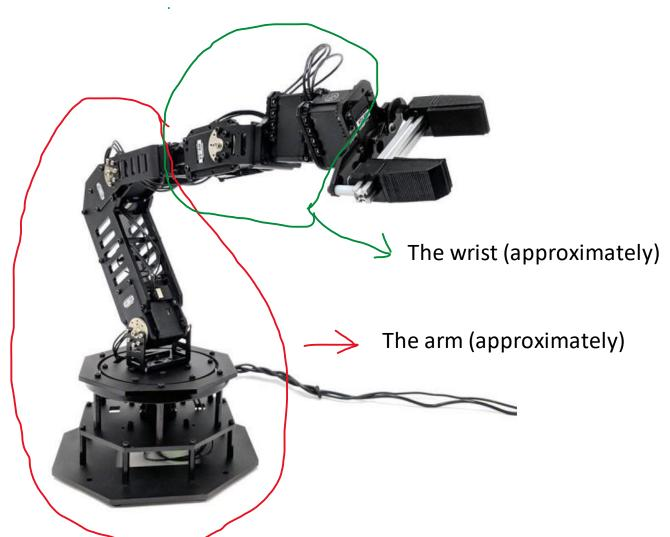
You will normally work with 2-4 DOF manipulators in the course. The wrist **by itself** is usually 3DOF. A "complete" manipulator is usually 3DOF of the arm + 3DOF of the wrist = 6DOF.
