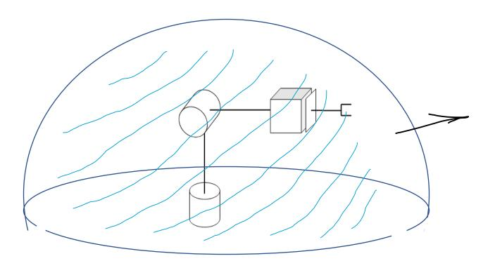
Workspace is a (half?)sphere, therefore a **spherical manipulator**
