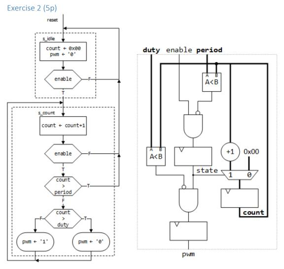
The ASMD diagram utilizes register operations for pwm and count, as indicated by their single arrow assignment " $\leftarrow$ ", thus the correct block diagram can be identified having registers for count, pwm in addition to the state registers (present in all state machines). After this assessment, the last wrong alternative can be identified by its excessive register usage, making the timing indicated in the diagram unachievable.
