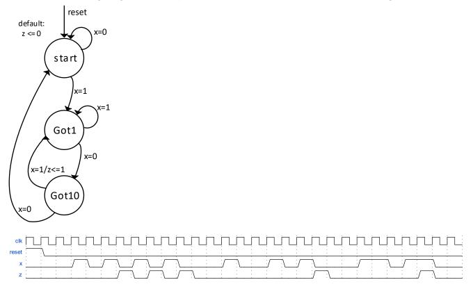
The 101 sequence detector will hoist the z flag for exactly one clock cycle, after the last '1' in a "101" sequence has been completed. Eg. the sequence of 00...01010110 will flag z as follows 00...000010100.
