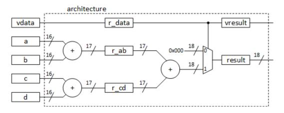
/2p Pipelining of v\_result <= rdata, rdata <= vdata (names can be anything) /2p r\_ab = a+b, r\_cd = c+d (or similar) /2p result = r\_ab + r\_cd when r\_data (eg. using mux or and)
