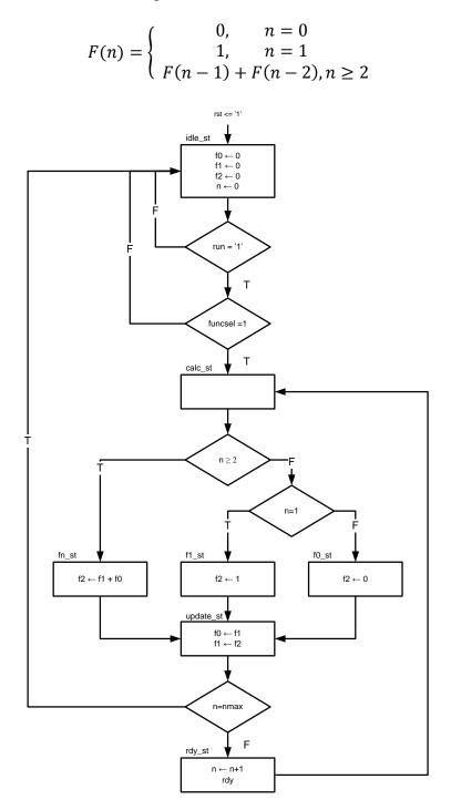
Implement the ASM-diagram above as a two-process state machine in synthesizable (RTL) VHDL. You must define your own additional internal signals after need. The Fibonacci state machine has the following entity:
