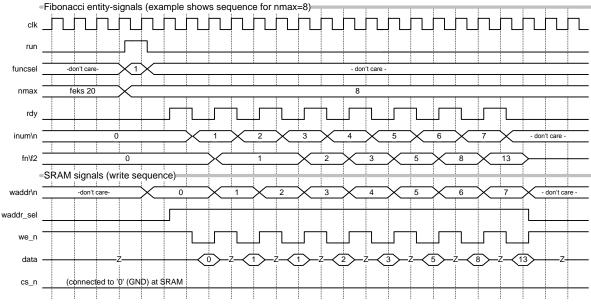
Please notice that the above timing diagram follows the timing of the state machine described in 11c)
