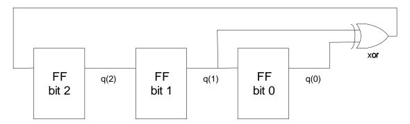
Note that an xor operation is executed between bit 0 and bit 1, and the result of xor is entered at the input of bit 2 in the 3-bit shift register.
