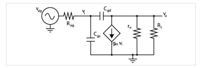
The illustration shows the small signal model of a CS gain stage. Given that  $g_m=1rac{\mathrm{mA}}{\mathrm{V}}, r_o||R_L=30\mathrm{k}\Omega, R_{sig}=4.8\mathrm{k}\Omega, C_{gs}=100\mathrm{fF}$  and the -3dB cut off is  $\omega_{-3\mathrm{dB}}=100\mathrm{Mrad}$ , what is the DC gain  $A_{DC}$  and  $C_{gd}$ ?
