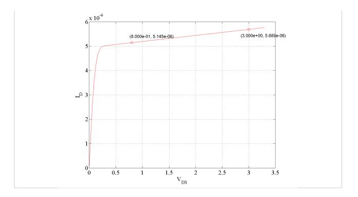
From the  $i_D$  vs  $v_{DS}$  graph shown and the marked points, compute the parameter  $\lambda$ .
