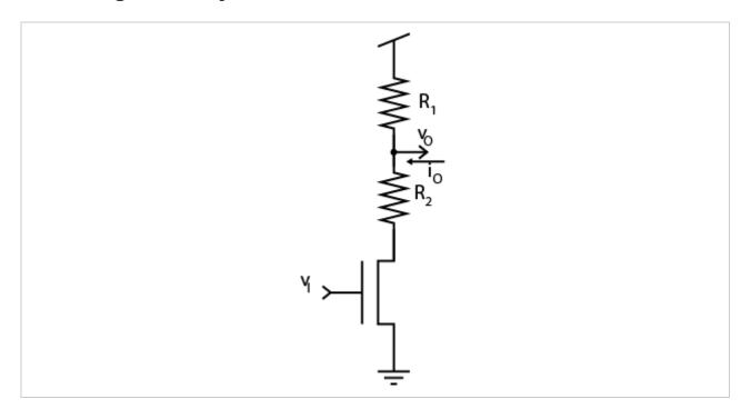
For the circuit in the schematics perform a small signal (!) analysis and find an expression for the total output resistance  $R_O=\frac{v_o}{i_o}$  and the total transconductance  $G_M=\frac{i_o}{v_i}$  and the gain  $A=\frac{v_o}{v_i}$ ! To form your expressions you may use the small signal variables  $g_m, r_o$  of the transistor as well as the resistors  $R_1, R_2$ . In other words express these terms as functions of those four variables (or a subset of them).
