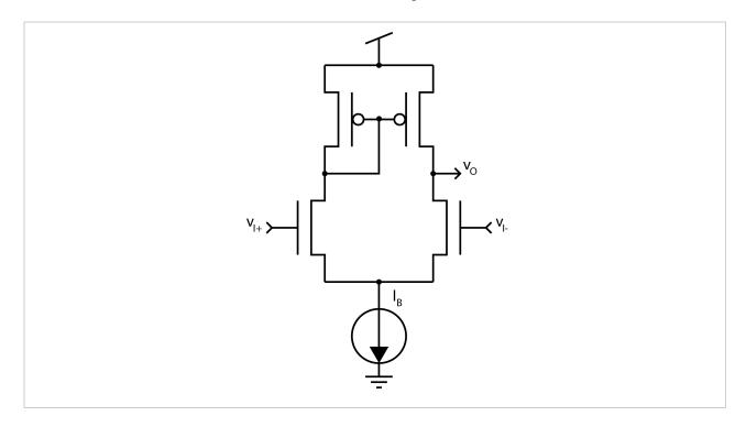
An nFET differetial pair is loaded with a pFET current mirror and an ideal current source provides a bias current  $I_B$  of 100 $\mu$ A (i.e. this is a current mirror loaded differential amplifier, see illustration). Compute its differential small signal gain  $A=\frac{v_o}{v_{i+}-v_{i-}}$  if  $k_n=k_n'\frac{W}{L}=500\mu\mathrm{A}$  and  $k_p=k_p'\frac{W}{L}=300\mu\mathrm{A}$  and the Early voltage  $V_A=\frac{1}{\lambda}=20\mathrm{V}$  for both type of transistors is.
