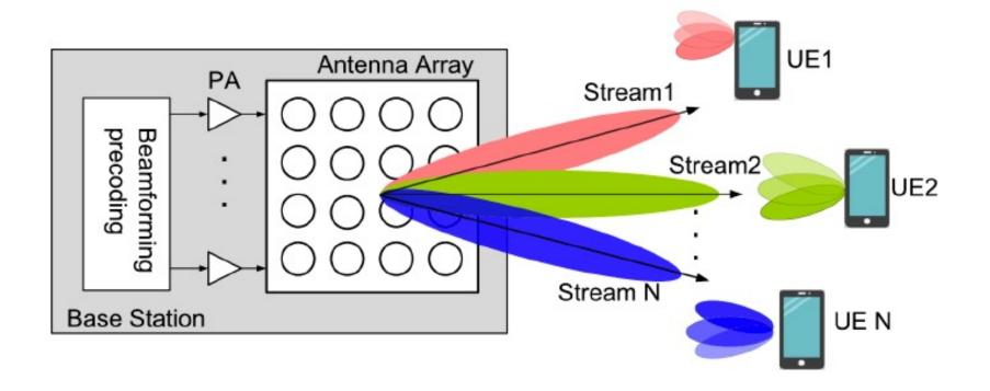
To address high attenuation, beamforming is used!
