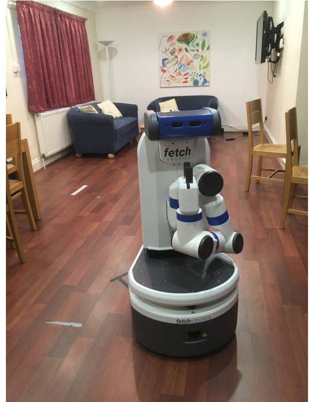
Figure 6. The Fetch Robot navigation stack was modified to provide slow in, slow out movement.
