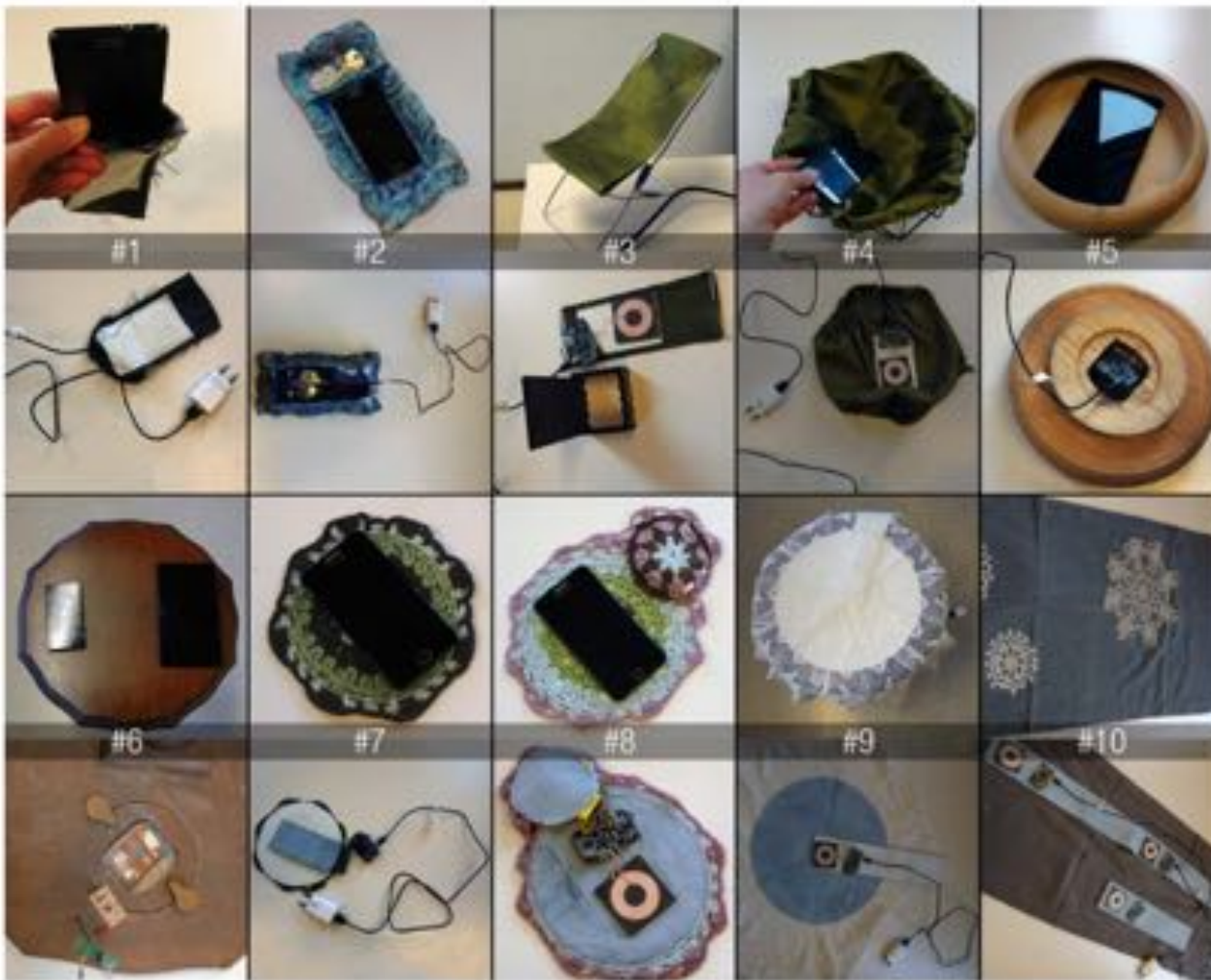
Figure 4: The 10 final designs manifested as functional prototypes. For each design of the two rows, the top image demonstrates the visible front of the design, while the bottom image reveals the underlying technical components.
