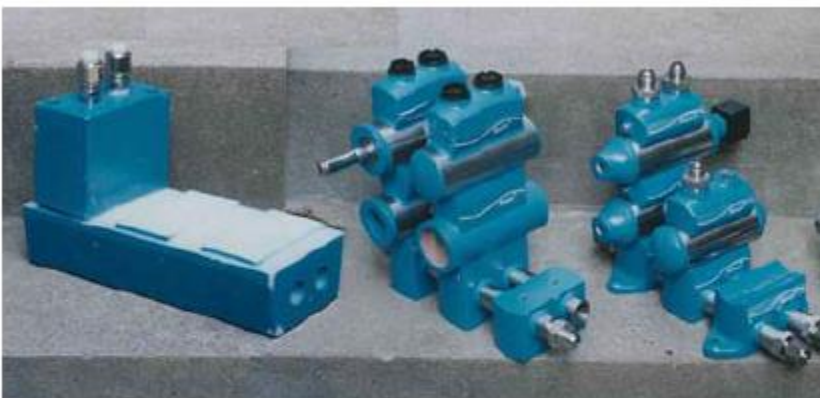
Fig. 6 Mock-ups of valves and manifolds from the WORM project. The mock-up to the left was from the second workshop, middle third workshop, and the mock-up with the most details to the right is from the fourth workshop
