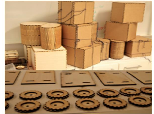
Figure 2. Top: Basic shapes. Bottom: Laser cut wheels
