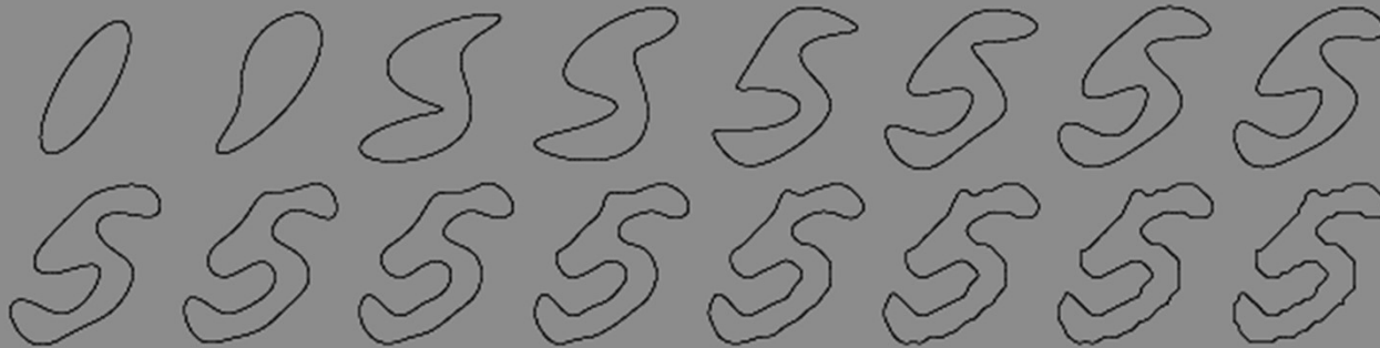
Figure 19: Character '5' reconstructed by elliptic Fourier descriptors of orders up to 1, 2, ... 10; 15, 20, 30, 40, 50, and 100, respectively.
