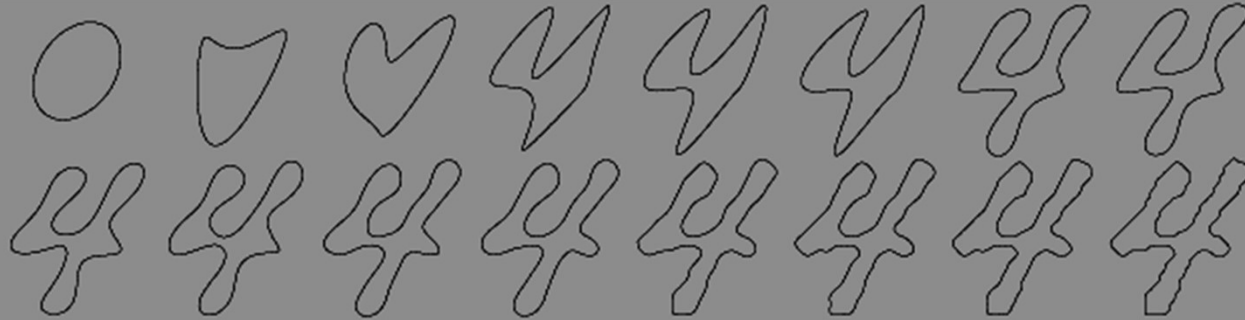
Figure 18: Character '4' reconstructed by elliptic Fourier descriptors of orders up to 1, 2, ... 10; 15, 20, 30, 40, 50, and 100, respectively.
