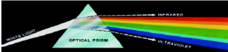
Figure 2-22. A qualitative illustration of chromatic refraction through a prism.
