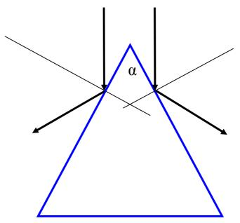
Two parallel beams of light are reflected off the two symmetric faces of the prism.
