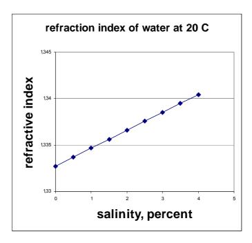
It increases approximately linearly from 1.33260 for pure water. The slope of the curve is 0.00195, and we make the assumption that this may be extrapolated linearly.
