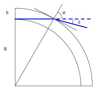
An object on the horizon is lifted by refraction by an angle  $\delta$ . Assuming vacuum outside a uniform atmosphere, Snell's law gives:
