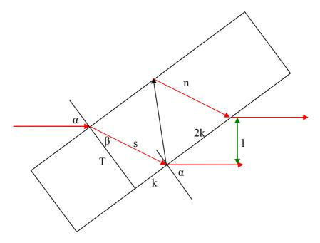
The twice reflected beam will be displaced relative to the first by an amount l, given in units of the thickness of the slab:
