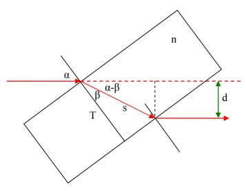
Let the angle of incidence be  $\alpha$ , while  $\beta$  is the angle of refraction as the beam enters the plane parallel slab. The index of refraction is n, and the thickness of the slab is T.
