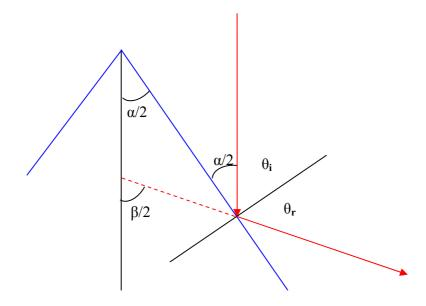
The angle of incidence  $\theta_i$  equals the angle of reflection  $\theta_r$  and the same is true for their 90° complements.
