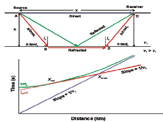
We consider a simple two-layer model as shown in the figure above, where the P-wave velocity of layer 1 and 2 is  $v_1$  and  $v_2$ , respectively (note  $v_2 > v_1$ ). In general, a receiver will measure three different wave contributions: direct wave, reflected wave and refracted wave.
