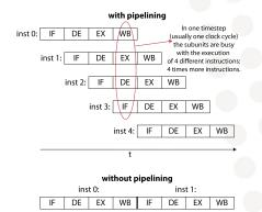
The pipeline in this example achieves a 4 times bigger instruction throughput. Note, though, that instruction 0 has the same *delay*. An 'annovance' are instructions that cause program counter jumps: then the execution of the pre-fetched instructions is interrupted and the pipeline restarted.
