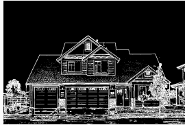
(a) 3x3 Sobel gradient magnitude, T = 10\% of max
