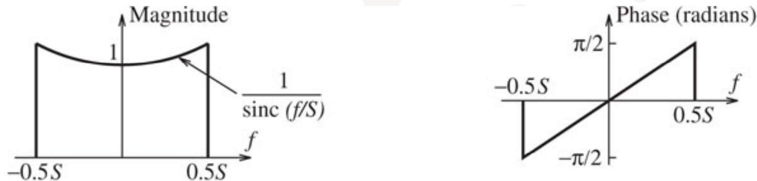
FIGURE 7.10 Spectrum of a filter that compensates for sinc distortion. To undo its effects, the filter gain is chosen as the reciprocal of the sinc (in the principal range). The filter is chosen to have linear phase
