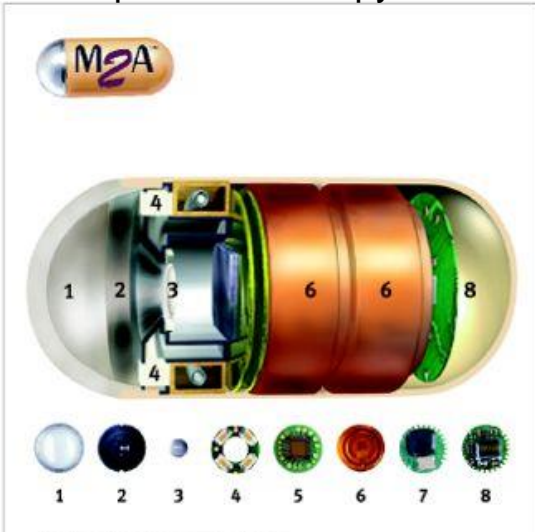
VECTOR-Versatile Endoscopic Capsule for gastrointestinal TumOr Recognition
