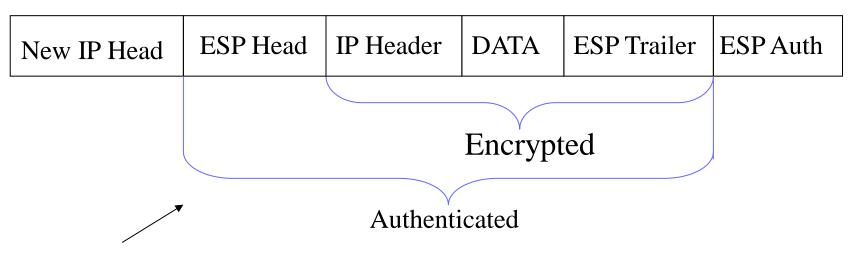
Original IP Packet protected by Tunnel-ESP
