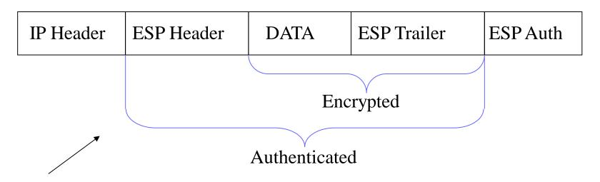
Original IP Packet protected by Transport-ESP
