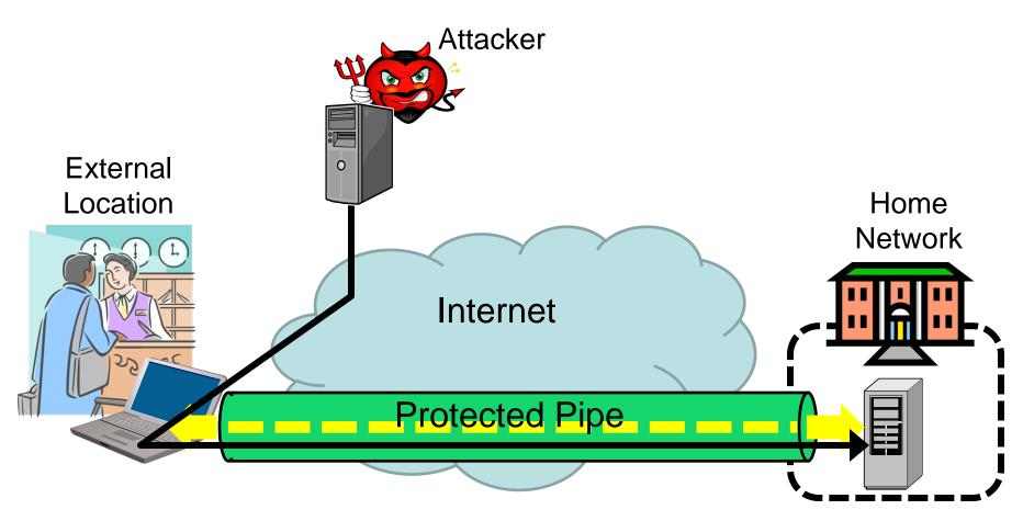
Secure pipe can be attack channel to home network!
