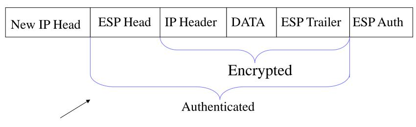
Original IP Packet protected by Tunnel-ESP
