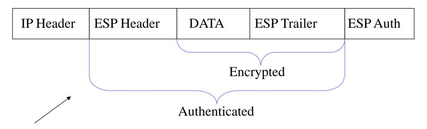
Original IP Packet protected by Transport-ESP
