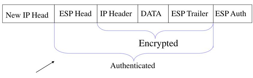
Original IP Packet protected by Tunnel-ESP
