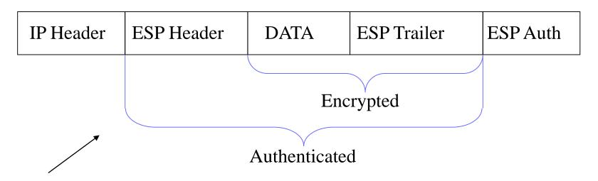
Original IP Packet protected by Transport-ESP
