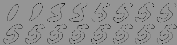
Figure 19: Character '5' reconstructed by elliptic Fourier descriptors of orders up to 1, 2, ..., 10; 15, 20, 30, 40, 50, and 100, respectively.
