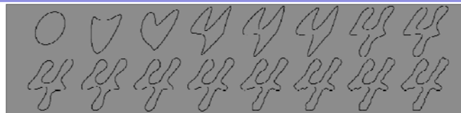
Figure 18: Character '4' reconstructed by elliptic Fourier descriptors of orders up to 1, 2, ..., 10; 15, 20, 30, 40, 50, and 100, respectively.
