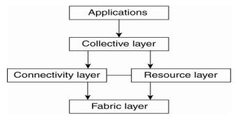
A layered architecture for grid computing systems.
