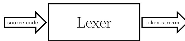
Figure 2.1: Input and output of a lexer
