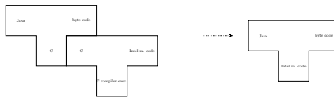
Figure 1.9: Composition of T-diagrams: compiling compiler code
