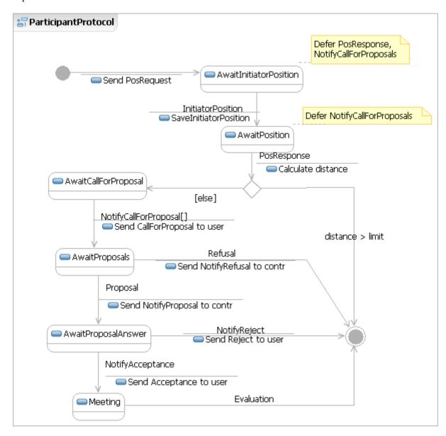
When this state machine begins, the first thing we need to do is to determine the user's position by sending a PosRequest. Next, we await three pieces of information: the Initiator's position, this user's position and the call-for-proposal details. By using the defer mechanism, we can ensure that these signals are handled in a sensible order. Only if the user is sufficiently close to the initiator, will the negotiation continue and the call-for-proposal is forwarded to the user.
