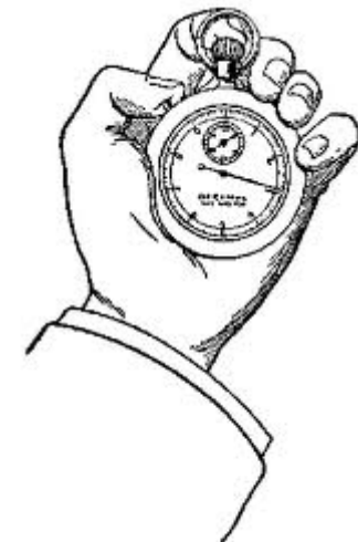
FIGURE 4.—STOP WATCH WITH DECIMAL FACE
