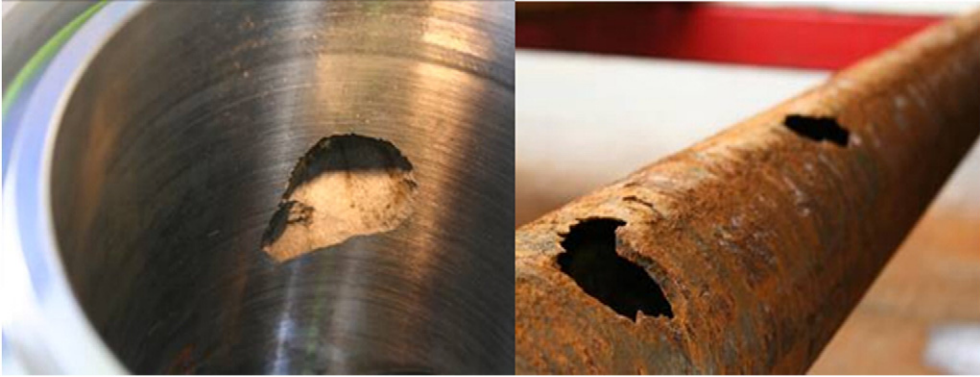
Fig. 2. Illustrations of corrosion in of a well's tubing.
