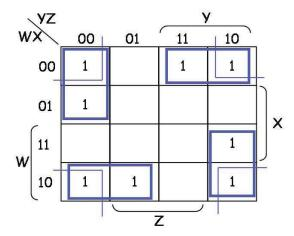
$F = \bar{W}\bar{Y}\bar{Z} + \bar{W}\bar{X}Y + W\bar{X}\bar{Y} + WY\bar{Z}$
